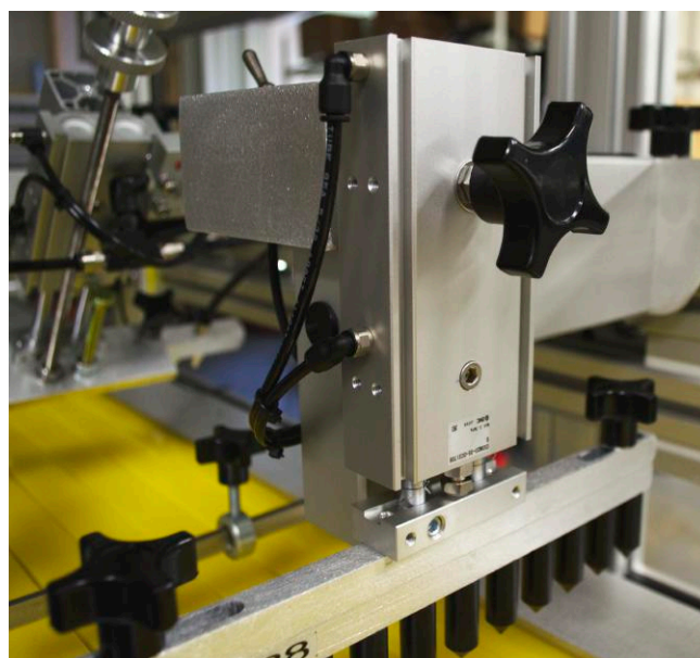
Figure 15. Dibble cylinder and lock handle (flat cylinder attached to upright assembly arm). Dibbling bar and pins with both locking handles are directly under cylinder unit.
