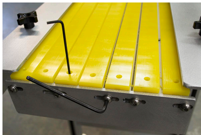
Figure 22. Unscrewing UHMW bed to rotate rails for even wear.
