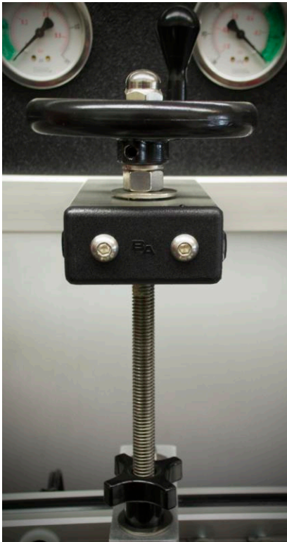
Figure 8. Height adjust arm with lower locking handle and upper adjusting handle.
