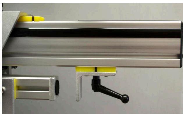
Figure 6. Stroke assembly showing gap between handle bar and bumpers.
