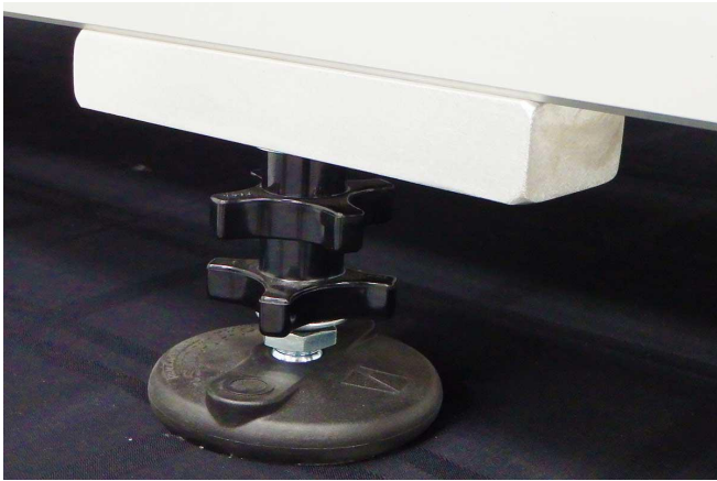
Figure 4. One of four leveling pads located at each outside corner of base of machine.
