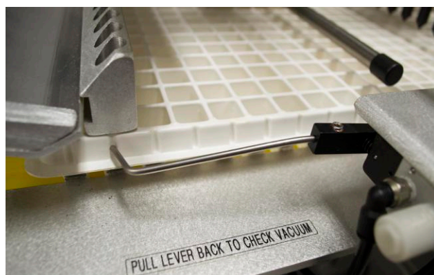
Figure 7. Tray is properly set up with first cell directly under drop tube, indexing push bar is set to forward wall of cell. In the foreground is the stainless steel vacuum actuator
