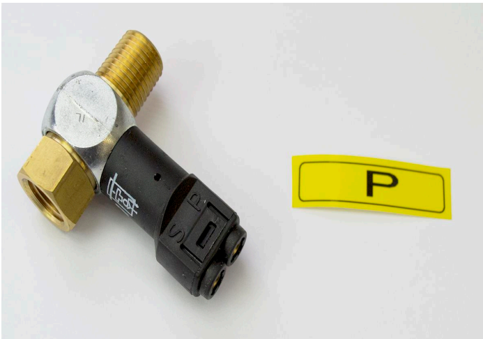
Figure 19. New sensor showing S & P airline sections and "P" label.
