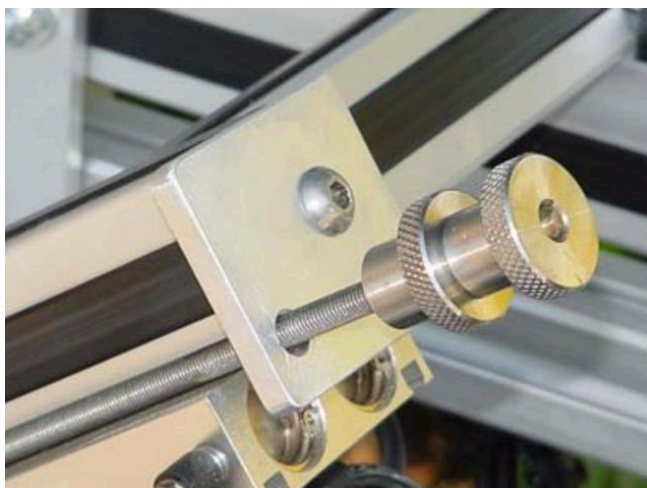
Figure 3. Two thumb screws to adjust height of the needle bar.
