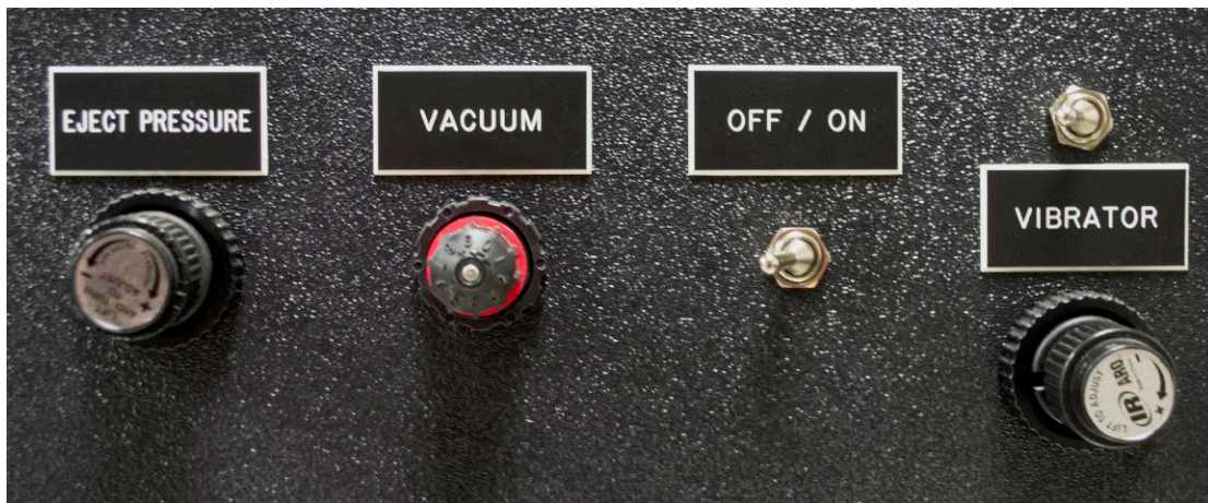
Figure 12. Eject pressure knob, vacuum knob, on/off switch, and vibrator switch/control knob.
